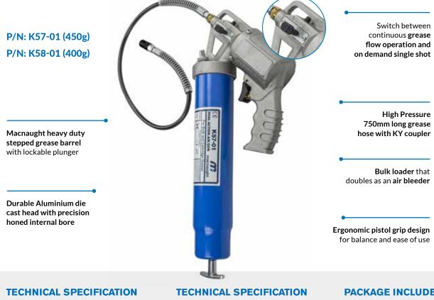
P/N: K57-01 Grease Capacity: 450g Ratio: 45:1 Output Pressure: Up to 6000psi Continous Delivery: Up to 400g/m On Demand Single Shot: 0.9g Air Inlet Pressure Range: 40 - 120psi Air Inlet: 1/4"F
